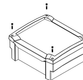
Fix the lid BCD\_OT-F-\_ using 4 screws.
