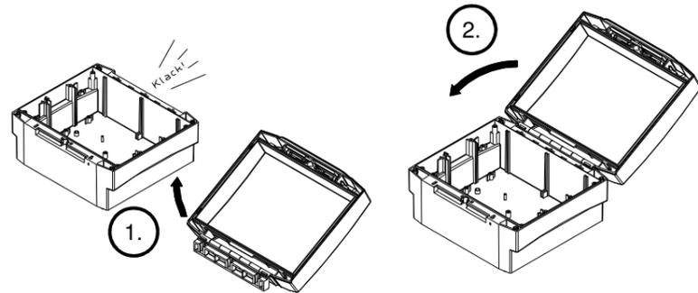
Snap the hinge onto the base (UT) (1.). Then close the lid (OT-G-\_) by swivelling it (2.).
