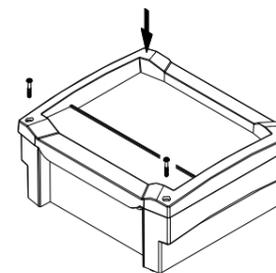
Place front frame BCD\_FO-K-\_ in position, clamp it in 2 places and screw it to the terminal compartment.
